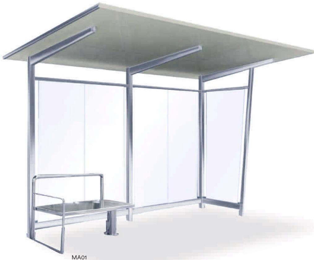
Pillars and bench in shiny, polished AISI-304 stainless steel. Roof panel with three 80 x 80mm support pillars for its fixing, with squares and horizontal profiles for glass enclosure. Galvanised and pre-lacquered injected polyurethane roof. Laminated safety glass. Supplied in kit form, with accessories and assembly instructions. Recommended anchoring: Embedded in the ground. Optional: Without MA01 side, with two MA01/2 sides. Customised glass.
