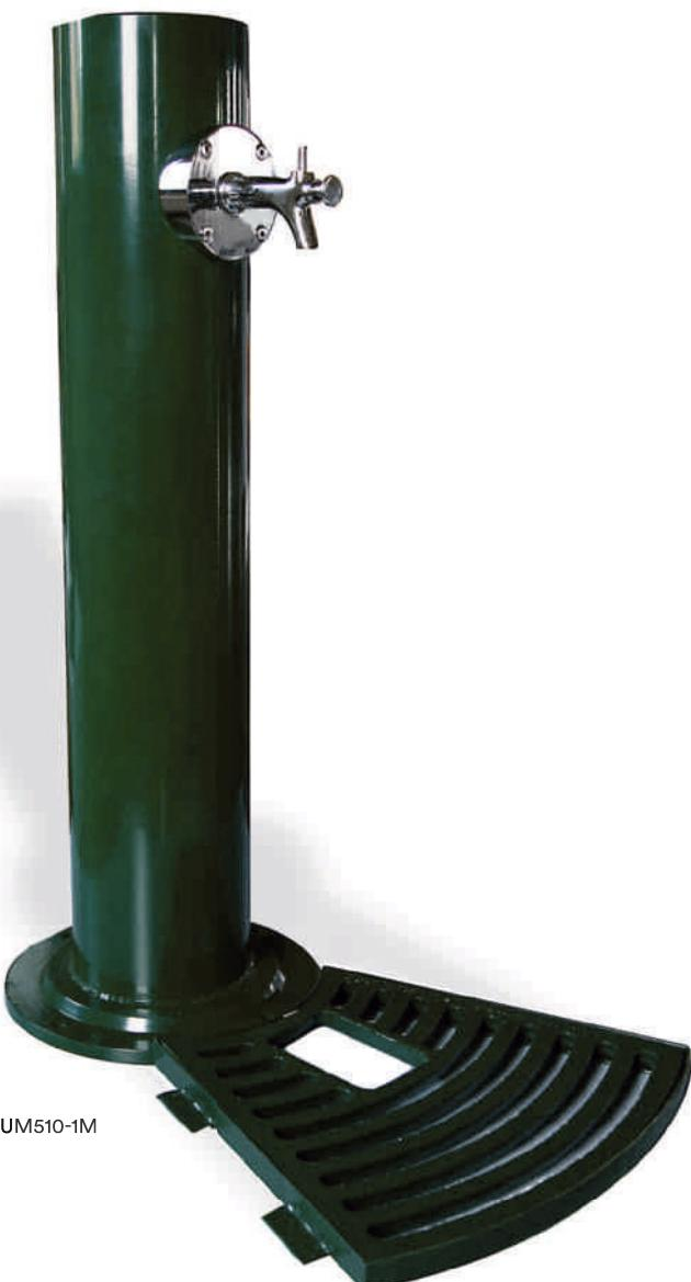
**Ø190 mm** steel body treated with Ferrus, a protective process for iron that guarantees high resistance to corrosion. Epoxy primer and green RAL 6005 polyester powder coated paint finish. Base with support and drain grate in ductile cast iron. Push button tap (UM510G) with nickel-plated steel support.
