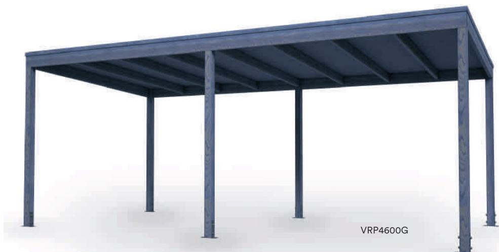
6000 × 3000 self-supporting gable roof pergola, made from European Oregon (Douglas) pinewood. 90 × 90 pillars, 170 × 45 beams, 140 × 45 joists and 115 × 21 tongue-and-groove boards. Lasur coating, 100% natural plant oil- and resin-based varnish finish, with a protective UV overcoat in grey colour. Asphalt roof (asphalt shingles) in autumn brown colour. Stainless steel fasteners and hot-galvanised steel anchors. Individual assembly kit. Optional: VRP4600 (lasur golden oak colour)
